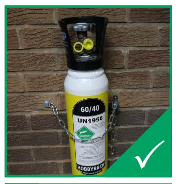
Ensure that cylinders remain upright and secured by using restraints, ratchet straps or chains
